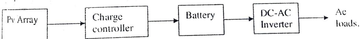
Fig 1 : Block Diagram of solar energy-operated inverter
