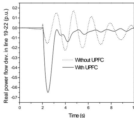
Figure 5. Real power flow in line 22-19 of Nigerian grid system.
