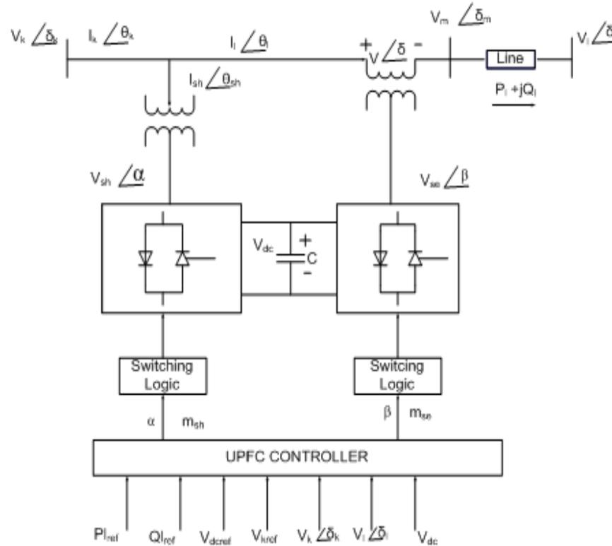
Figure 1. Block Diagram of a UPFC
