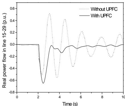
Figure 4. The damping effect of UPFC on the power flow in line 15-29.
