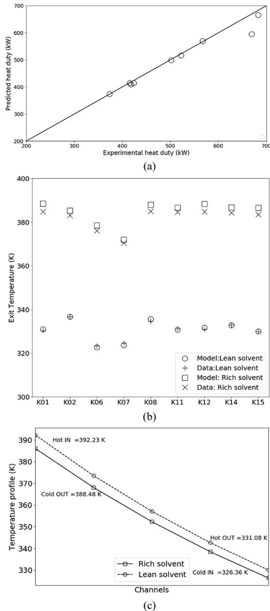
Figure 2: (a) Parity plot for the PHE heat transferred, (b) Exit temperature with plant data, (c) Temperature profile across the channels for case K01
