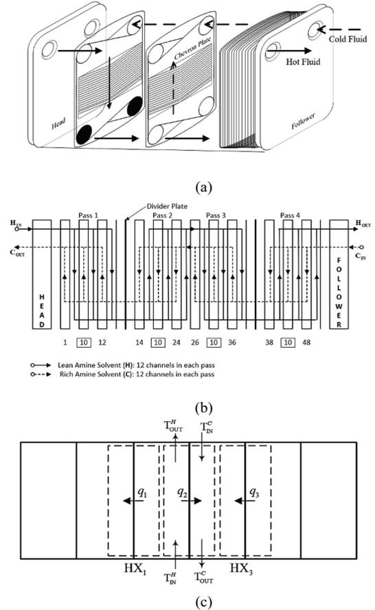
Figure 1: (a) Typical PHE layout (b) 4-pass-4-pass PHE with 12 channels for each pass and (c) sub-heat exchangers in a pass
