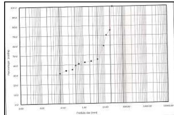
**Figure 4:** Particle Size Distribution Curve for BH/PIT-4
