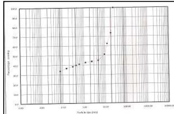
**Figure 3:** Particle Size Distribution Curve for BH/PIT-3
