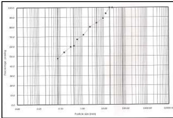
**Figure 6:** Particle Size Distribution Curve for Trial Pit-2
