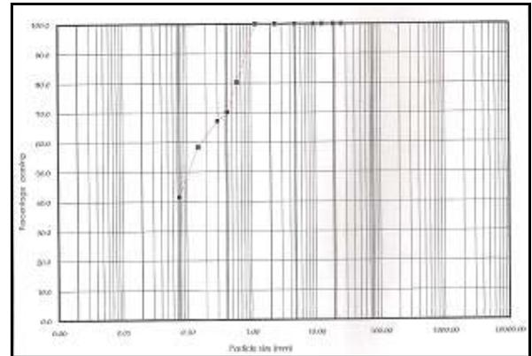
**Figure 8:** Particle Size Distribution Curve for Trial Pit-4
