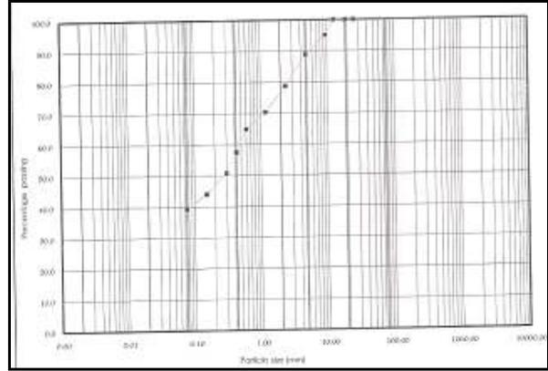
**Figure 7:** Particle Size Distribution Curve for Trial Pit-3
