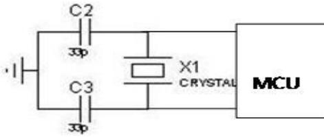
Figure 3.0: Crystal Resonator XT Configuration
