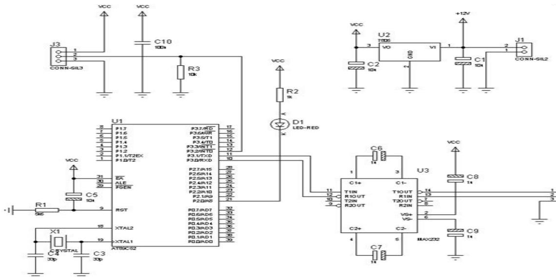
Figure 7.0: Card reader overall circuit diagram
