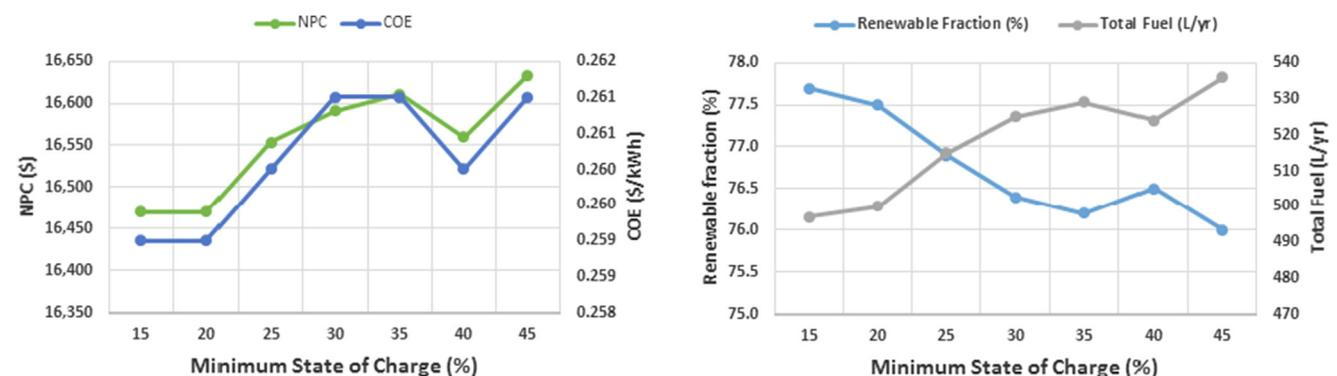
Fig. 16 The effect of varying the battery SOC<sub>min</sub> on the system costs, fuel, and renewable penetration.
