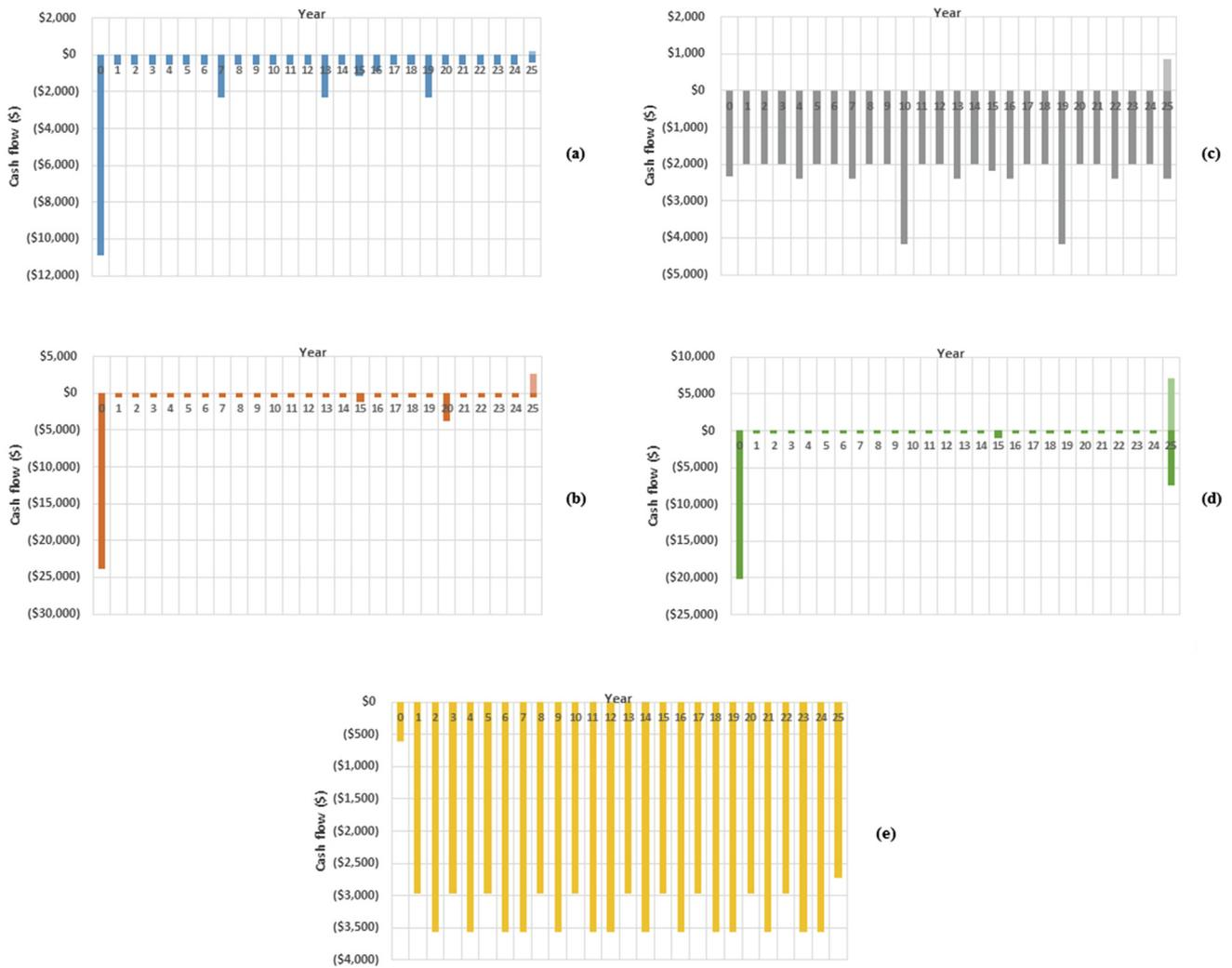
Fig. 12 Nominal cash flow results for different system cases. (a) Case 1: PV/DG/battery model (b) Case 2: PV/wind/battery model (c) Case 3: DG/battery model (d) Case 4: PV/battery model (e) Case 5: DG-only model (Current situation).
