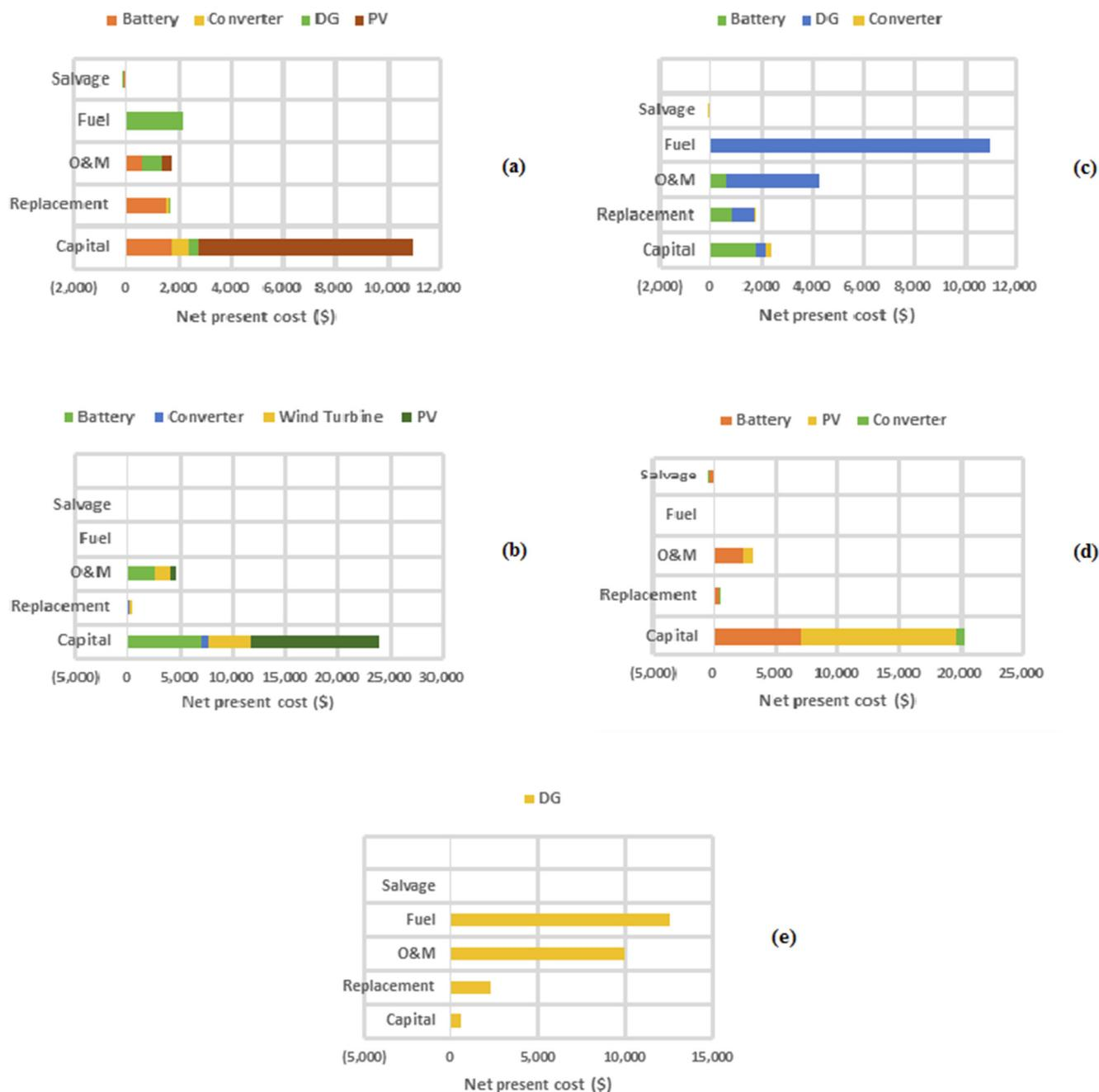
**Fig. 10** Cost summary of different system cases. (a) Case 1: PV/DG/battery model (b) Case 2: PV/wind/battery model (c) Case 3: DG/battery model (d) Case 4: PV/battery model (e) Case 5: DG-only model (Current situation).
