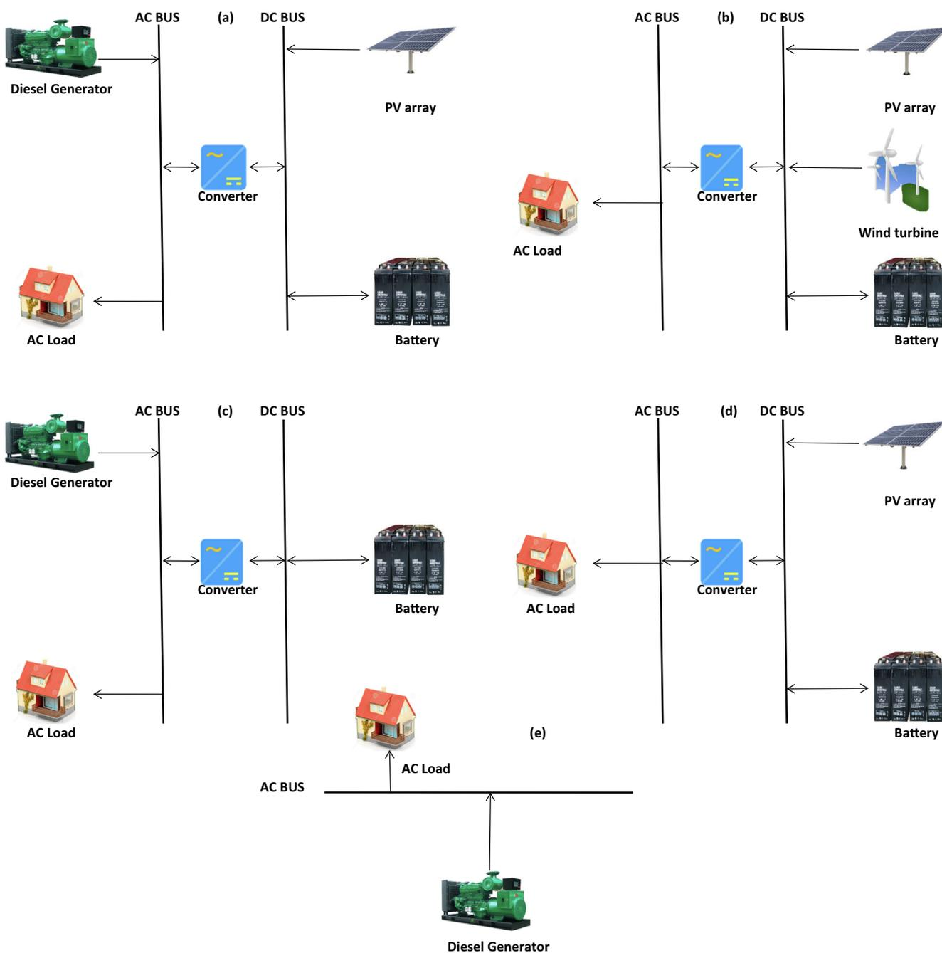
**Fig. 7** The schematic diagram of (a) Case 1: PV/DG/battery model (b) Case 2: PV/wind/battery model (c) Case 3: DG/battery model (d) Case 4: PV/battery model (e) Case 5: DG-only model.
