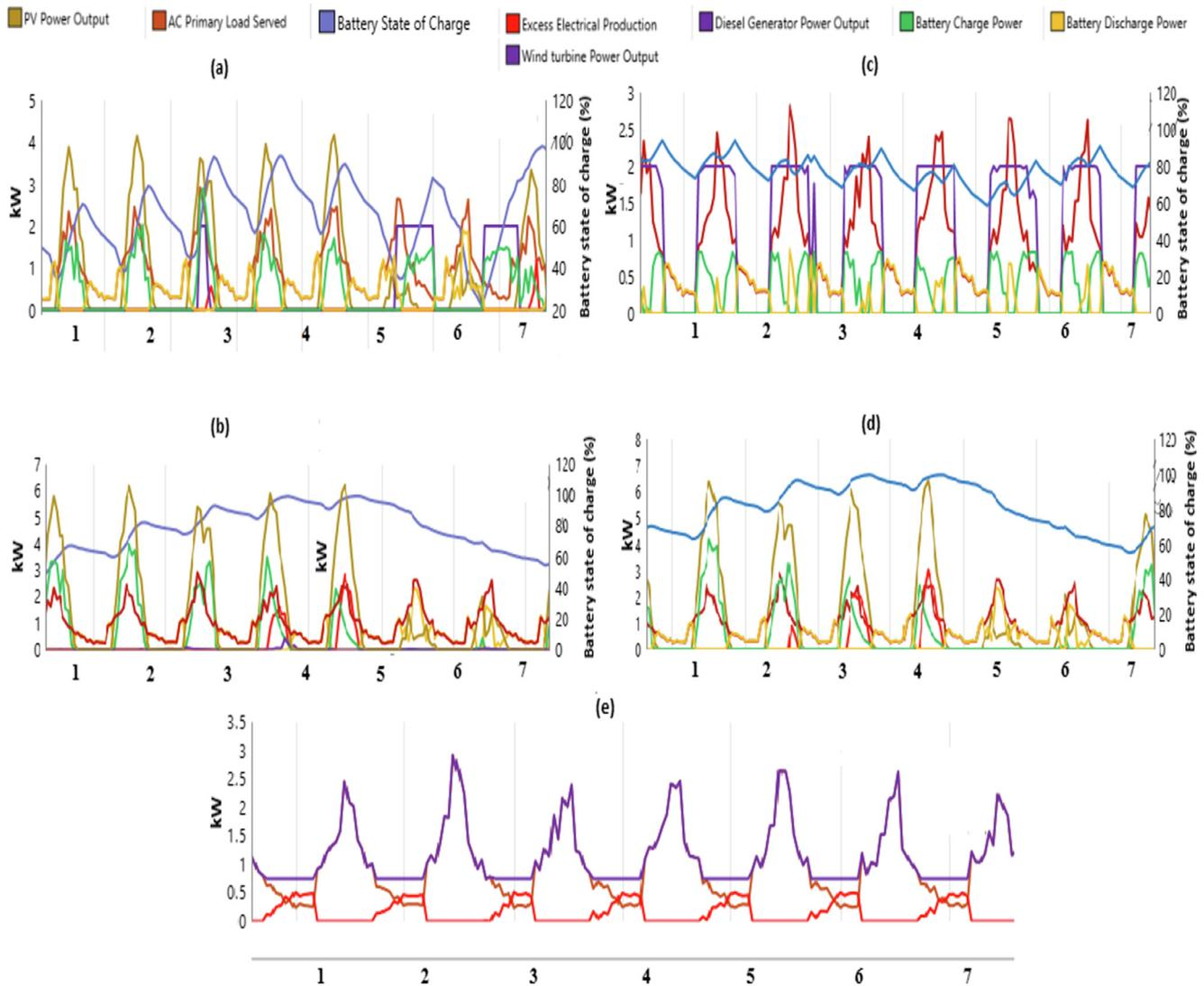
**Fig. 9** Power balance and battery state of charge of different system cases. (a) Case 1: PV/DG/battery model (b) Case 2: PV/wind/battery model (c) Case 3: DG/battery model (d) Case 4: PV/battery model (e) Case 5: DG-only model.
