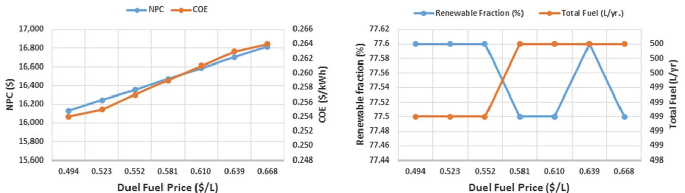
**Fig. 13** Effect of varying the fuel price on the system costs, fuel, and renewable penetration.
