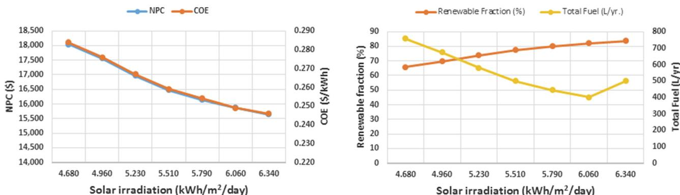
Fig. 15 Impact of varying solar radiation on system costs, fuel, and renewable penetration.
