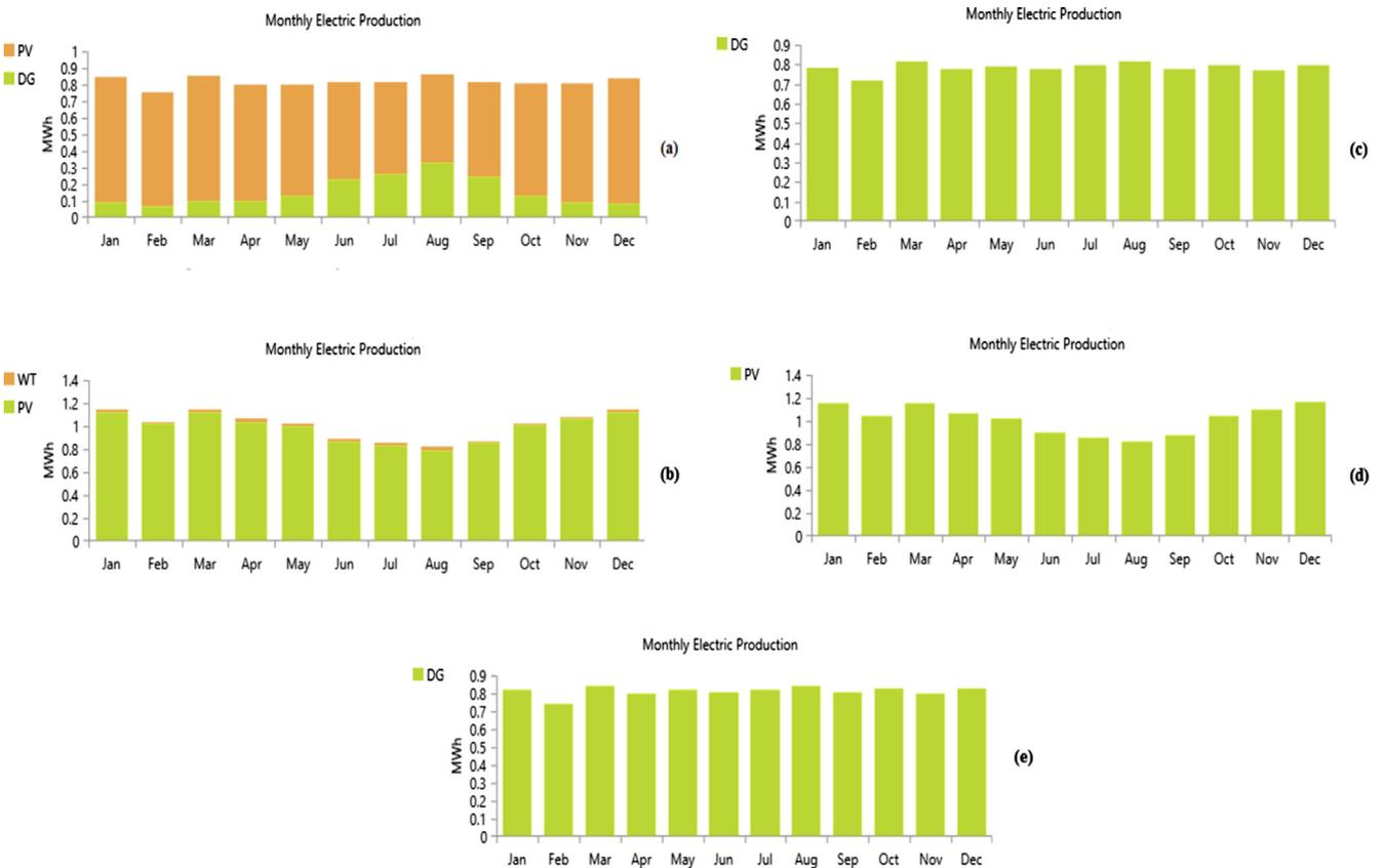
**Fig. 8** Monthly electric power production for different cases. (a) Case 1: PV/DG/battery model (b) Case 2: PV/wind/battery model (c) Case 3: DG/battery model (d) Case 4: PV/battery model (e) Case 5: DG-only model (Current situation).
