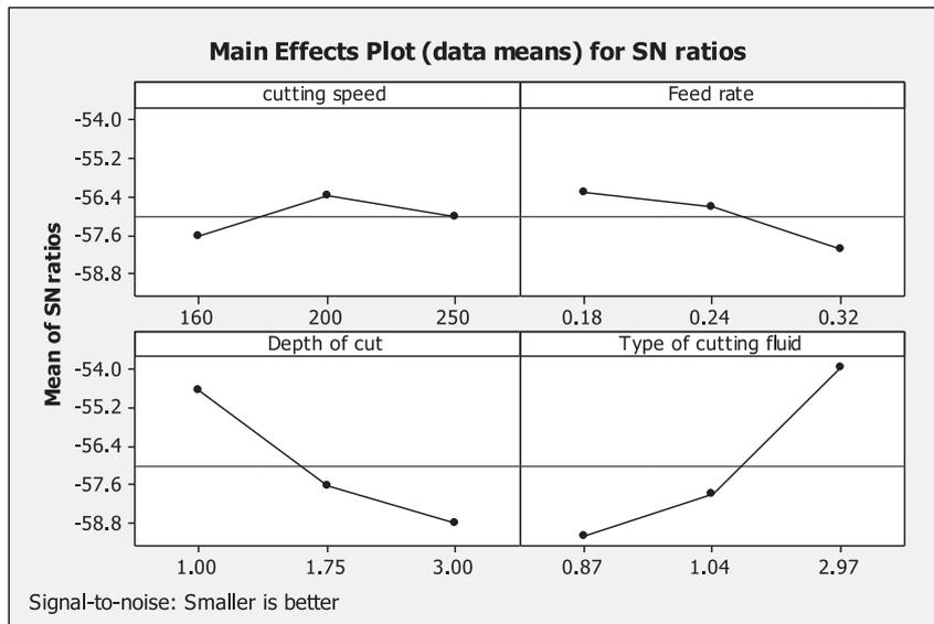
Fig. 7. Main effects plot of SN ratios for main cutting force.
