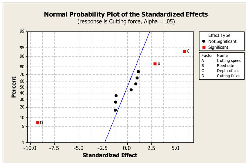
Fig. 9. Normal probability plot for cutting force.
