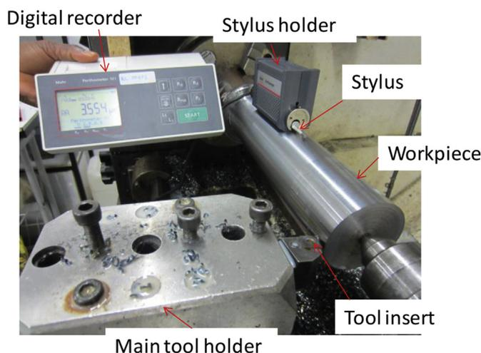
Fig. 3. Set up for surface roughness measurement.
