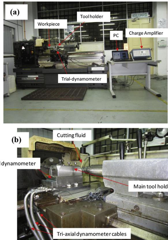
Fig. 2. Experimental set up for turning process.
