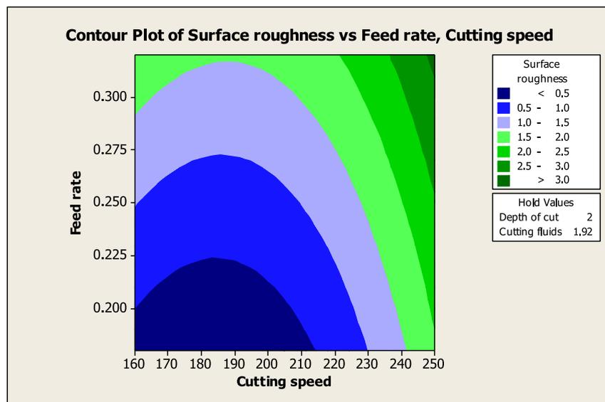
Fig. 5. Contour plots for surface roughness (Feed rate vs Cutting speed).
