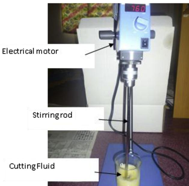
Fig. 1. Mixing with mechanical overhead stirrer.
