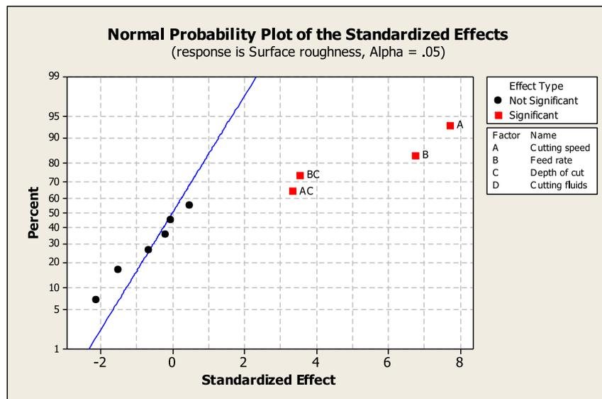
Fig. 6. Normal probability plot for surface roughness.
