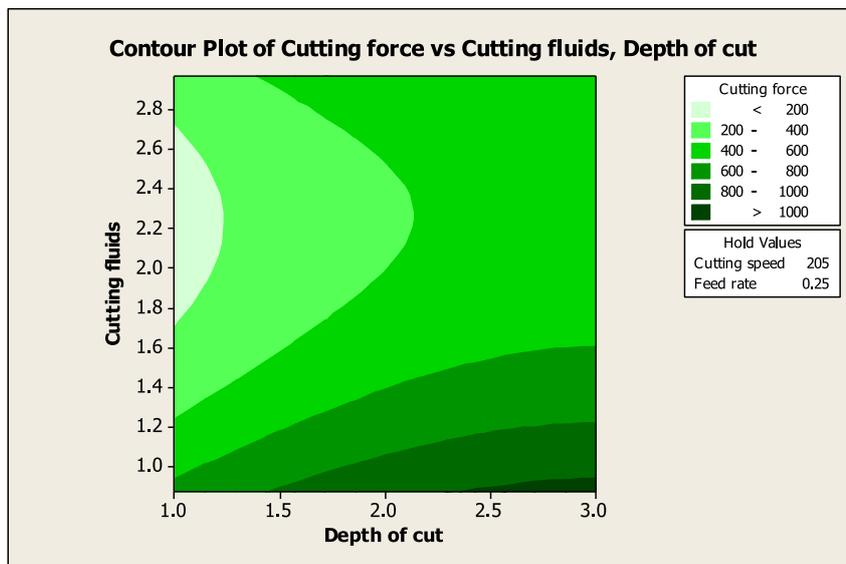
Fig. 8. Contour plots for cutting force (cutting fluid vs depth of cut).
