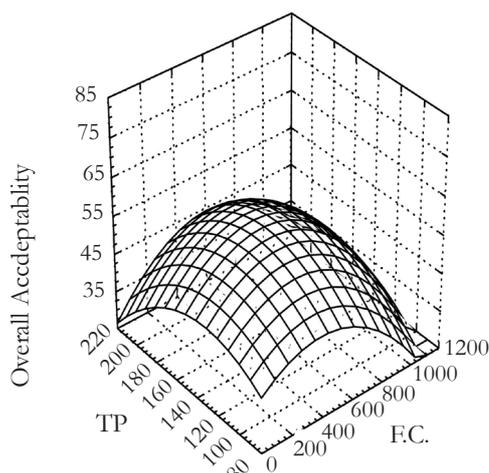
**Fig. 2:** Response surface plot of the effect of feed composition (FC) and barrel temperature (TP) on extrudate texture
