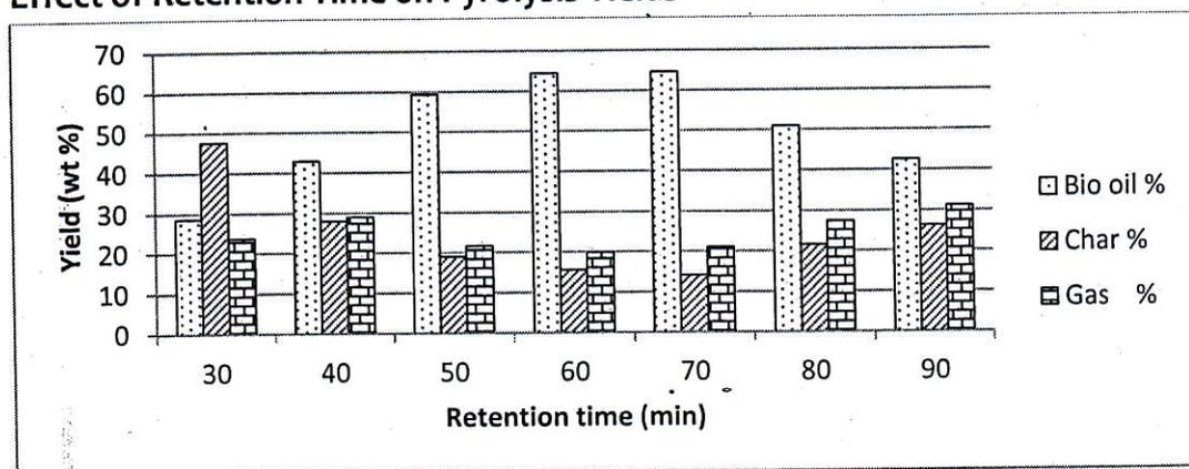
Chart 1- Products distribution as a function of retention time at a temperature of 600 °C, N<sub>2</sub> gas flow rate at 5L/min and feed particle size of 1.7 mm.
