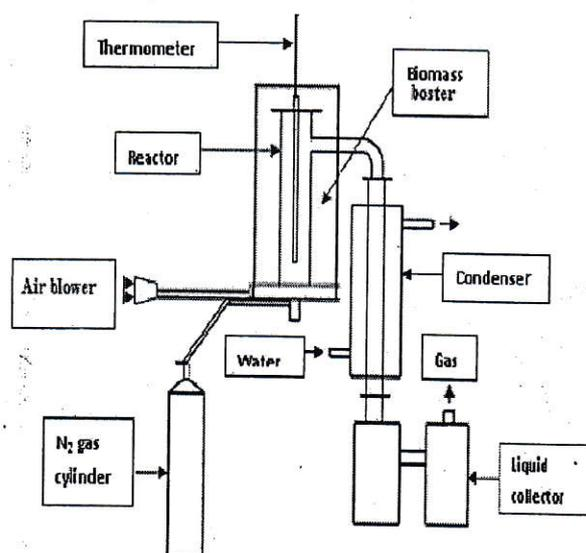
Figure 1: Schematic diagram of a fast pyrolysis setup
