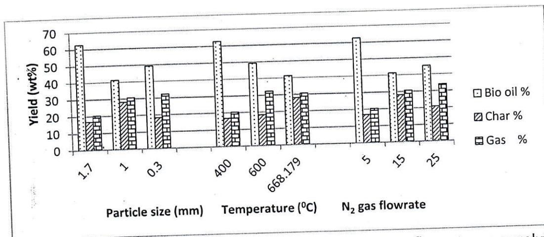
Chart 2: Effect of Particle size, Temperature and N<sub>2</sub> gas flowrate on pyrolytic products Yield
