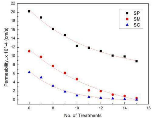
Figure 1:Hydraulic conductivity of treated soil
