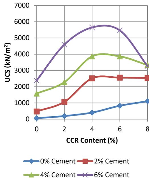
Figure 6: Variation of unconfined compressive strength with various dosages of cement and CCR after 28 days curing period
