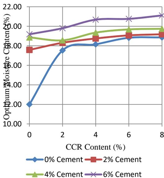
Figure 2: Variation of OMC with increase dosage of cement and CCR
