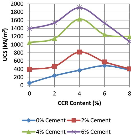
Figure 3: Variation of unconfined compressive strength with various dosages of cement and CCR after 1 day curing period
