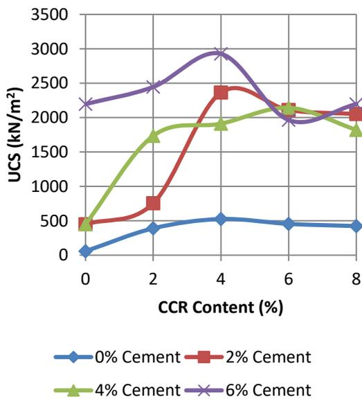
Figure 4: Variation of unconfined compressive strength with various dosages of cement and CCR after 7 days curing period
