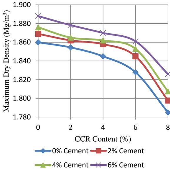
Figure 1: Variation of MDD with increase dosage of cement and CCR
