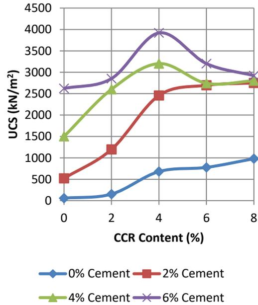
Figure 5: Variation of unconfined compressive strength with various dosages of cement and CCR after 14 days curing period
