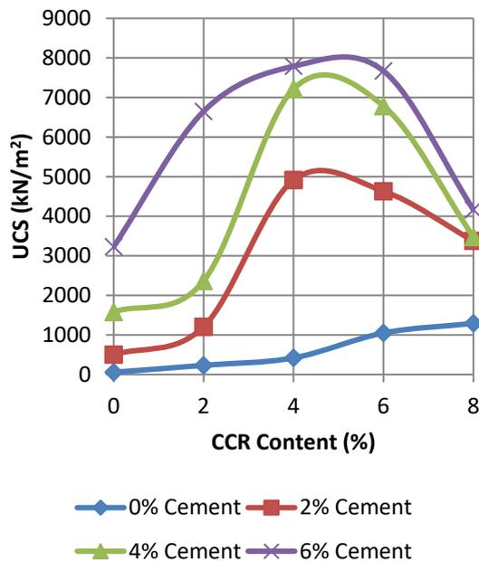
Figure 7: Variation of unconfined compressive strength with various dosages of cement and CCR after 60 days curing period
