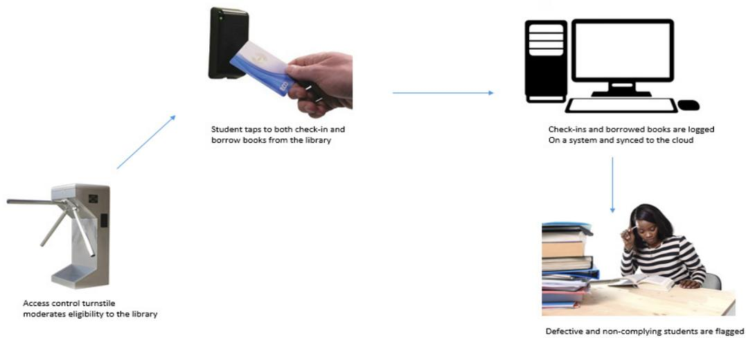
**Figure 2: Flow process of the Sanwo's campus and Library RFID based application**
