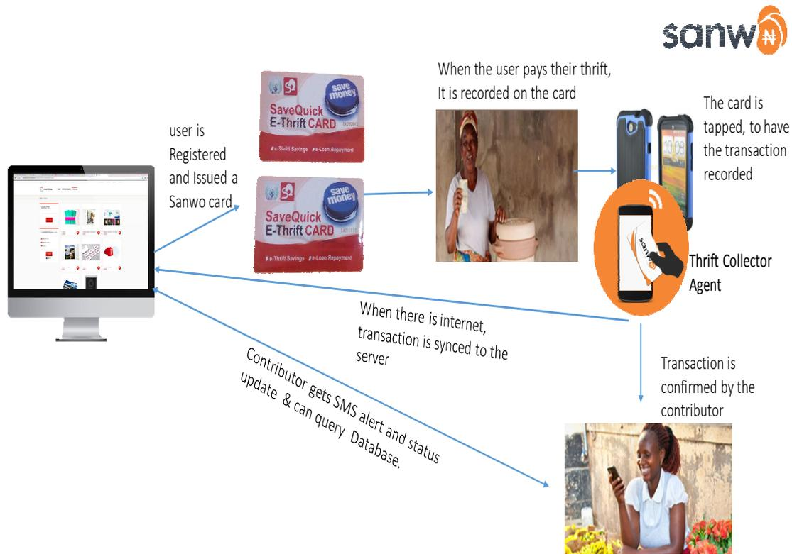
**Figure 3: Electronic Thrift Collection Flow process of offline RFID based application**
