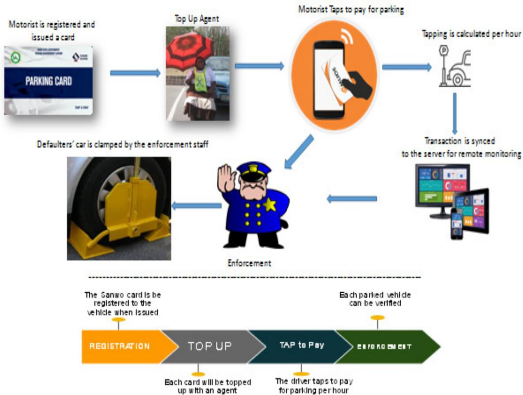
**Figure 4: RFID Based Offline Vehicle Parking Fee Collection Flow Process**
