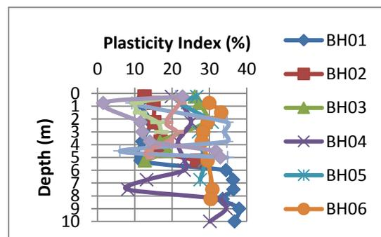
FIGURE 7: VARIATION OF PLASTICITY INDEX WITH DEPTH
