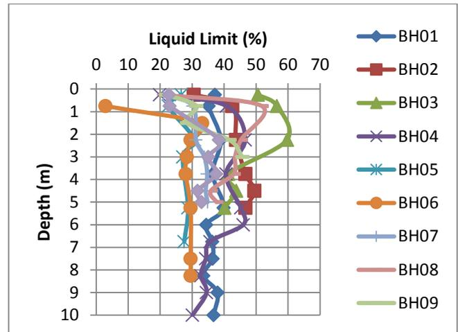
FIGURE 5: VARIATION OF LIQUID LIMIT WITH DEPTH
