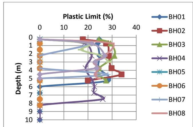
FIGURE 6: VARIATION OF PLASTIC LIMIT WITH DEPTH
