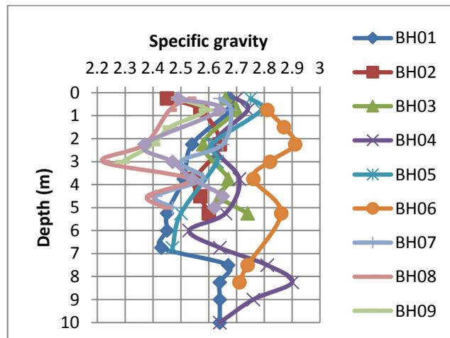
FIGURE 4: VARIATION OF SPECIFIC GRAVITY WITH DEPTH
