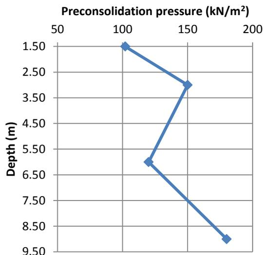
FIGURE 6: VARIATION OF PRECONSOLIDATION PRESSURE WITH DEPTH AT BH 5
