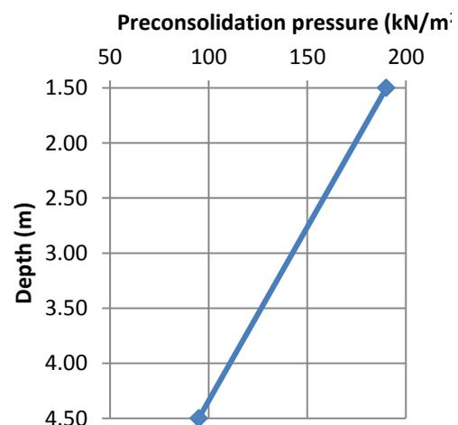
FIGURE 5: VARIATION OF PRECONSOLIDATION PRESSURE WITH DEPTH AT BH 4
