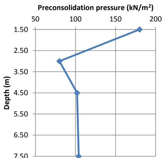
FIGURE 7: VARIATION OF PRECONSOLIDATION PRESSURE WITH DEPTH AT BH 6
