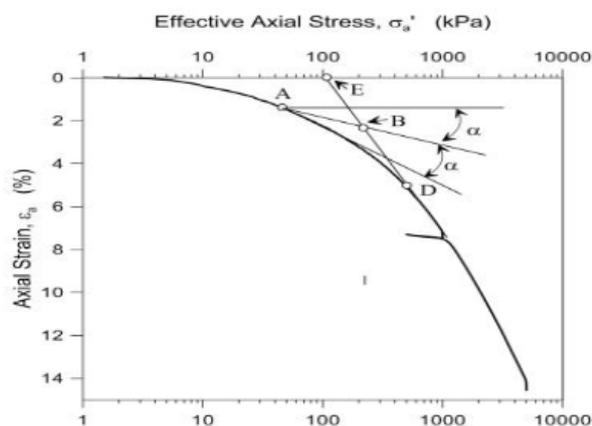
FIGURE 1: CASAGRANDE METHOD OF EVALUATING PRECONSOLIDATION PRESSURE  $P_c$  (SOURCE: HOLTZ AND KOVACS, 1981)
