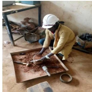
Fig. 3: Compaction test
