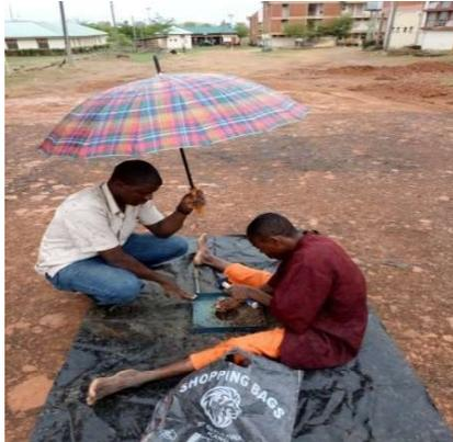
Fig. 10: In-situ density test on the road surface
