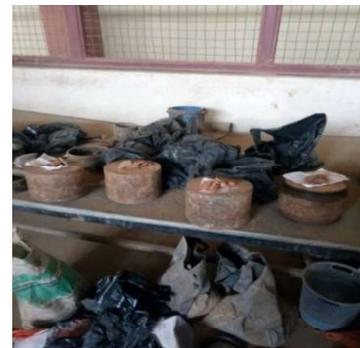
Fig. 4: Compacted samples for CBR test
