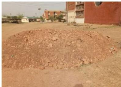
Fig. 1: Pile of lateritic soil
