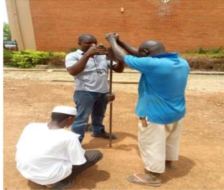
Fig. 11: DCP Test on a compacted surface
