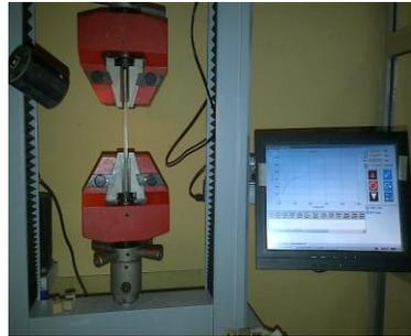
Figure 2: Bamboo splint in tension
