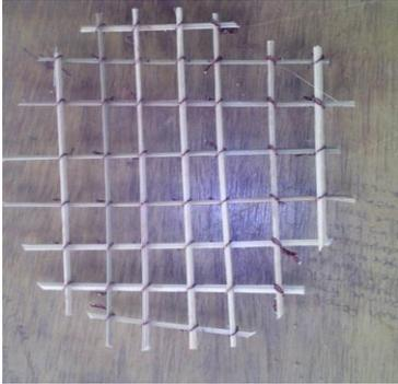
Figure 3: A typical layer of the bamboo reinforcement
