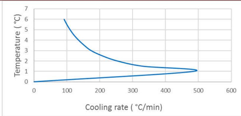
Figure 2b: Cooling rate curve of cast specimen cooled in mould immersed in ice block.
