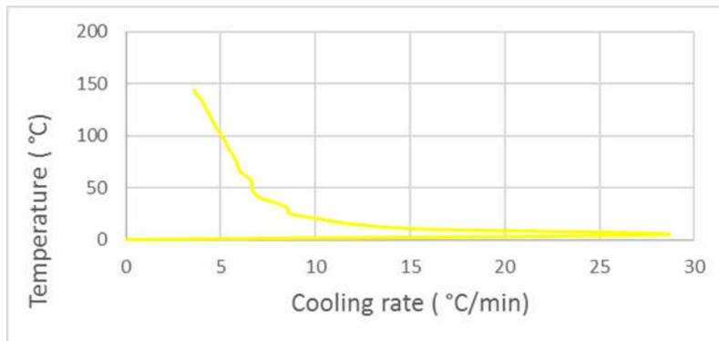
Figure 2d: Cooling rate of cast specimen cooled in mould at 230 °C.
