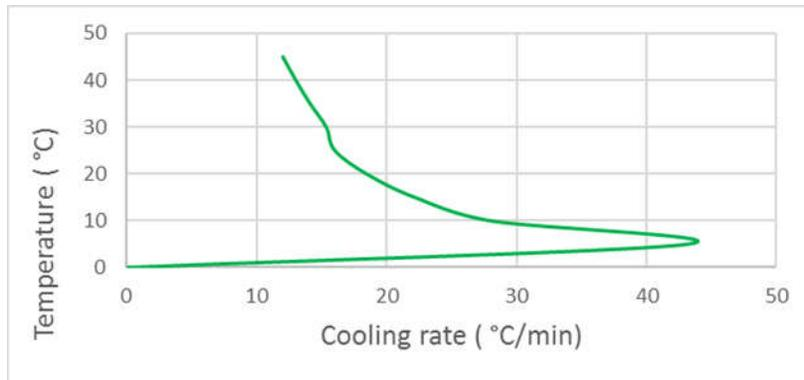
Figure 2a: Cooling rate curve of cast specimen cooled in mould at room temperature.
