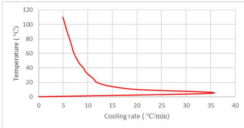
Figure 2c: cooling rate curve of cast specimen cooled in mould at 140 °C
