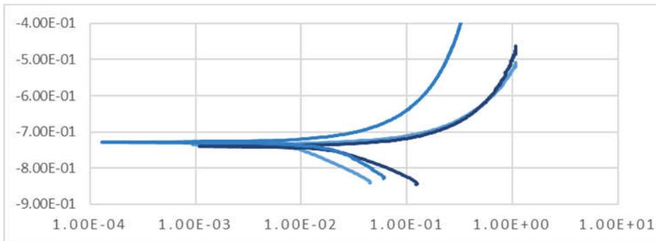
Figure 4a: Polarization curves from electrochemical tests of 6xxx aluminum alloy cooled in mould at room temperature.
