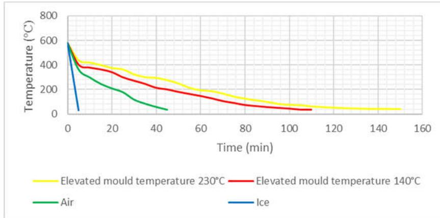
Figure 1: Cooling curves of 6xxx aluminum alloy under different mould temperature.
