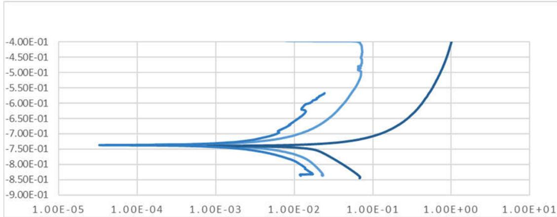
Figure 4c: Polarization curves from electrochemical tests of 6xxx aluminum alloy cooled in mould cooled at 140 °C.
