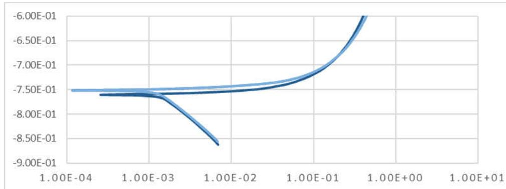
Figure 4b: Polarization curves from electrochemical tests of 6xxx aluminum alloy cooled in mould immersed in Ice block.
