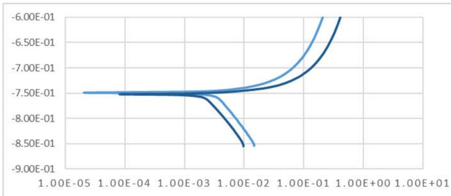
Figure 4d: Polarization curves from electrochemical tests of 6xxx aluminum alloy cooled in mould at 230°C.
