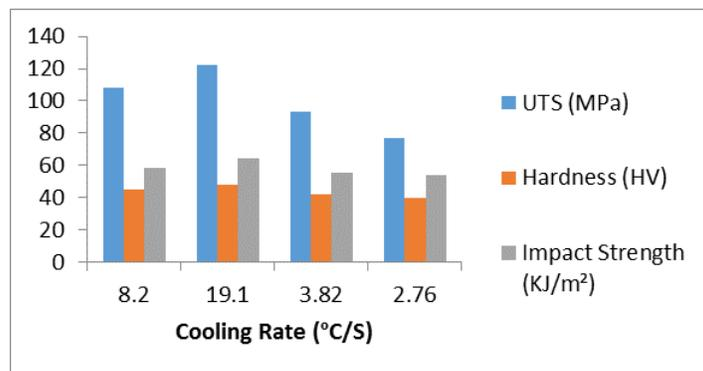
Figure 3: Variation in UTS, Hardness and Impact strength with cooling rate.
