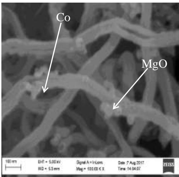
Fig. 2: HRSEM image of the as-synthesized CNTs showing Co and MgO Catalytic support
