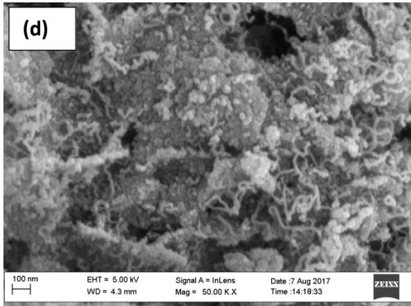
Fig. 5: HRSEM Micrograph of CNTs (a and b) represented the highest yield while (c and d) depicted the lowest yield CNTs at different magnification.
