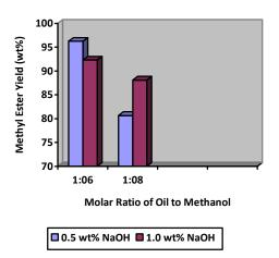
Fig 1. Effect of molar ratio of oil to methanol on the methyl ester yield at 90 minutes
