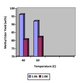
Fig 2. Effect of reaction temperature on methyl ester yield at 90 minute
