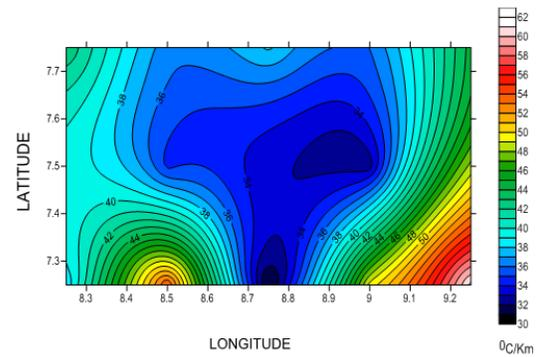
Figure 8, The geothermal gradient contour map of the study area
