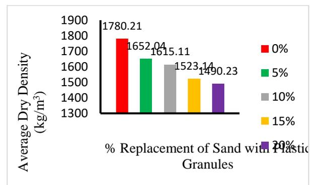
Figure 7: Dry Density of Concrete with Plastic Granules Partially Replaced Sand
