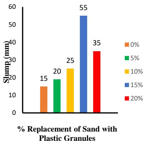
Figure 2: The Slump of Fresh Concrete
