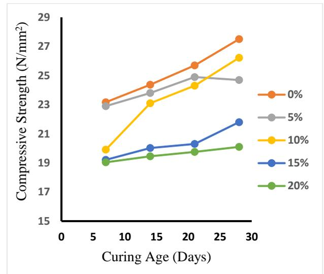
Figure 5: Compressive Strength with Curing age of Concrete with Plastic Granules Partially Replaced Sand.
