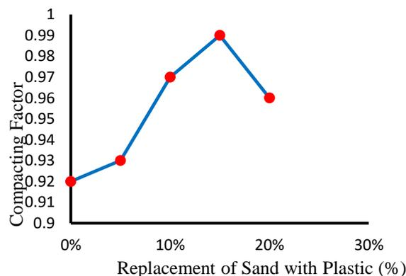
Figure 3: Compacting Factor of Concrete with Plastic Granules Partially Replaced Sand
