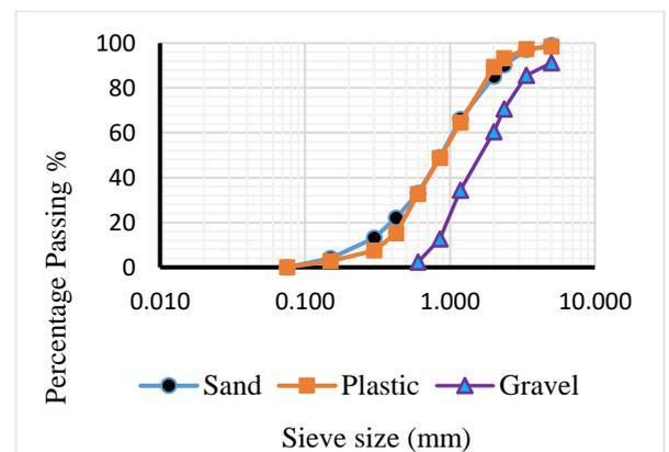
**Figure 1: Sieve Analysis for the Aggregates used**
