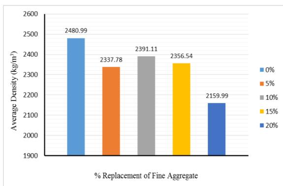
Figure 6: Bulk Density of Concrete with Plastic Granules Partially Replaced Sand
