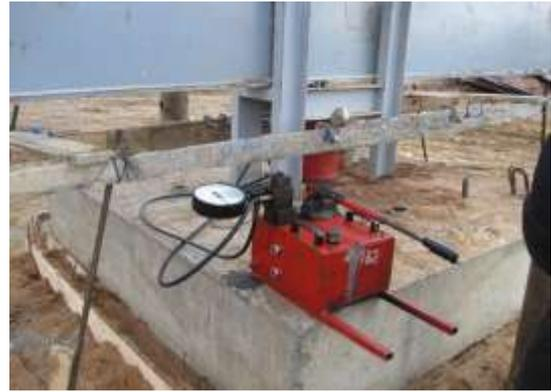
Fig.3: Hydraulic jack for field test loading
