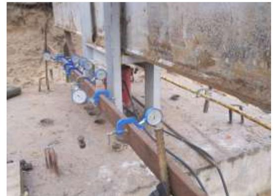
Fig. 4: Dial gauges for Settlement Reading
