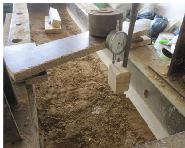
Figure 3. Settlement measurement on Dial gauge
