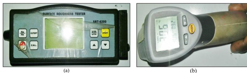
**Fig. 3.** Measuring equipment used during machining process (a) SRT surface roughness tester and (b) PeakTech infra-red thermometer.
