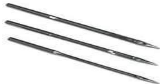
**Fig. 4.** Cryogenically treated sewing needles.
