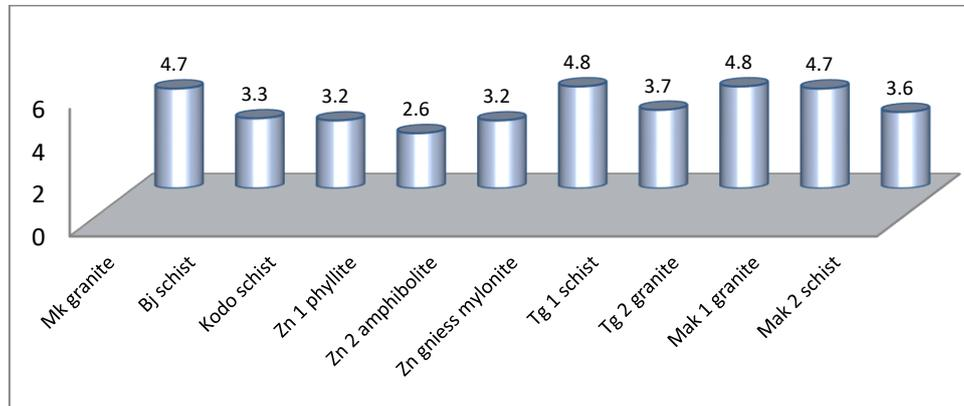
Figure 8: Weathering Intensity for study area (after Ruxton, 1968)
