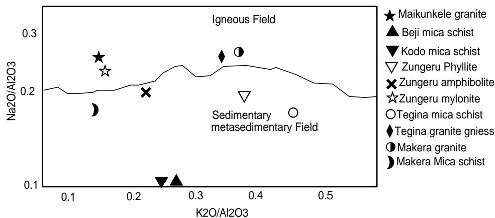
Figure 7: Na<sub>2</sub>O versus K<sub>2</sub>O plot for study area rocks (after Garrels and Mackenzie, 1971)
