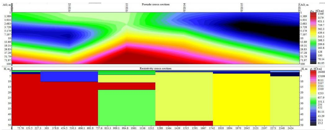
**Fig. 9. Pseudo cross-section and resistivity cross-section of profile 1 in the study area**
