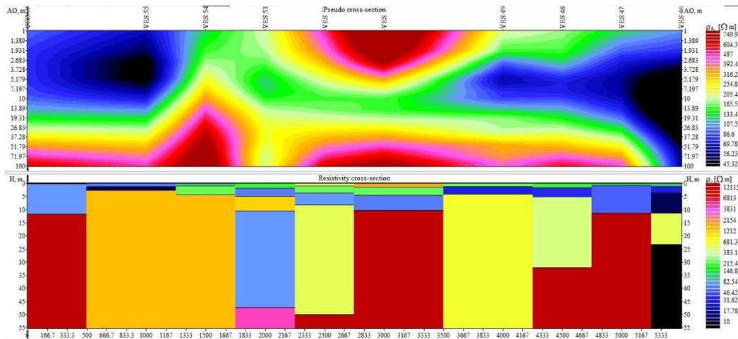
**Fig. 13. Pseudo cross-section and Resistivity cross-section of Profile 5 in the study area**
