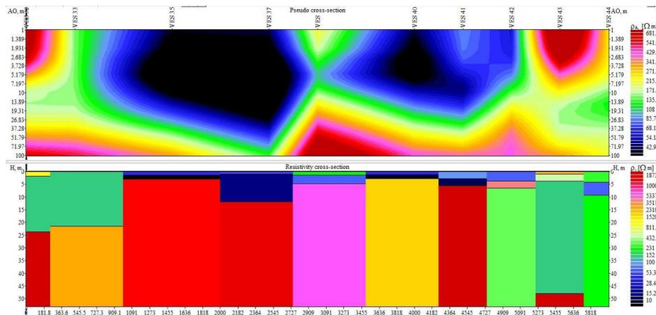
Fig. 12. Pseudo cross-section and Resistivity cross-section of Profile 4 in the study area
