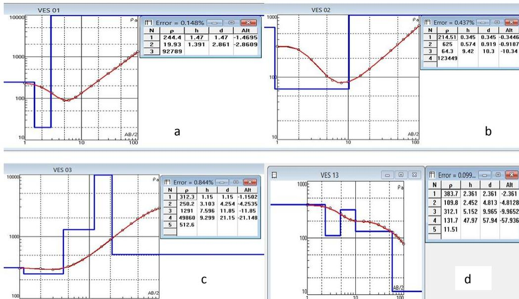
Fig. 8. Typical (a) H-Type curve, (b) HA – Type curve (c) and (d) other 5 – layer curve types
