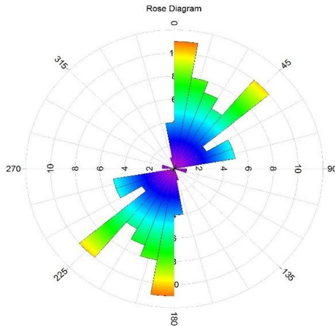
Fig. 7. Rosette diagram of joint directions
