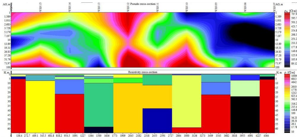
**Fig. 10. Pseudo cross-section and Resistivity cross-section of Profile 2 in the study area**
