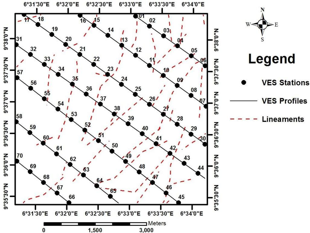
**Fig. 2. VES sounding stations along 7 Profiles (Profiles 1 to 7 from top to bottom). The spacing between VES sounding stations are 500 m apart.**
