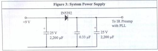
A diode is used as the decoupling element on the power supply in place of the normal R-C elements because it has a higher opposition to signal flow through the power rail. The 9 V DC was stabilized by a 2,200  $\mu F$  capacitor and fed to the power amplifier section directly—a decoupled version of 8.3 V was supplied to the IR amplifier and PLL.
