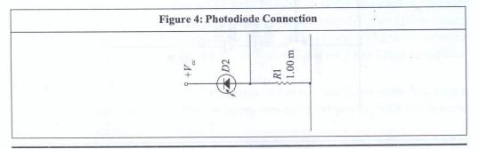
for 1 nW of incident light, the excitation current of the photodiode develops a voltage V across the 1 m $\Omega$  resistance. This voltage is amplified by a two-stage amplifier designed around the LM 358 (Figure 5).
