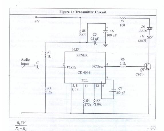
The audio signal was superimposed in the control voltage, thus causing the control voltage to vary in consonance with the audio signal, producing a frequency-modulated output. The square wave RF output was fed into the base emitter junction of a C9014 high frequency transistor (Figure 2).
