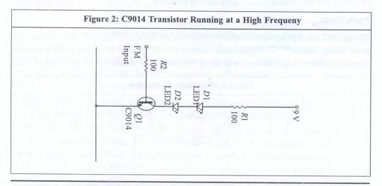
Two infrared emitters were used to radiate the generated FM wave. A current-limiting resistor of 100  $\Omega$  was inserted in series with the emitters. The value of resistance was calculated for a diode peak current of 0.05 A, as shown below:
