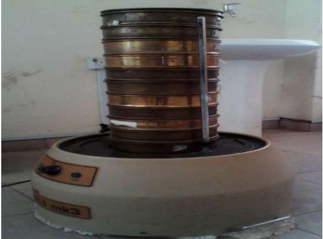
**Plate I: Sieve Analysis of Soil and Borehole samples in the laboratory (Amadi, 2010)**
