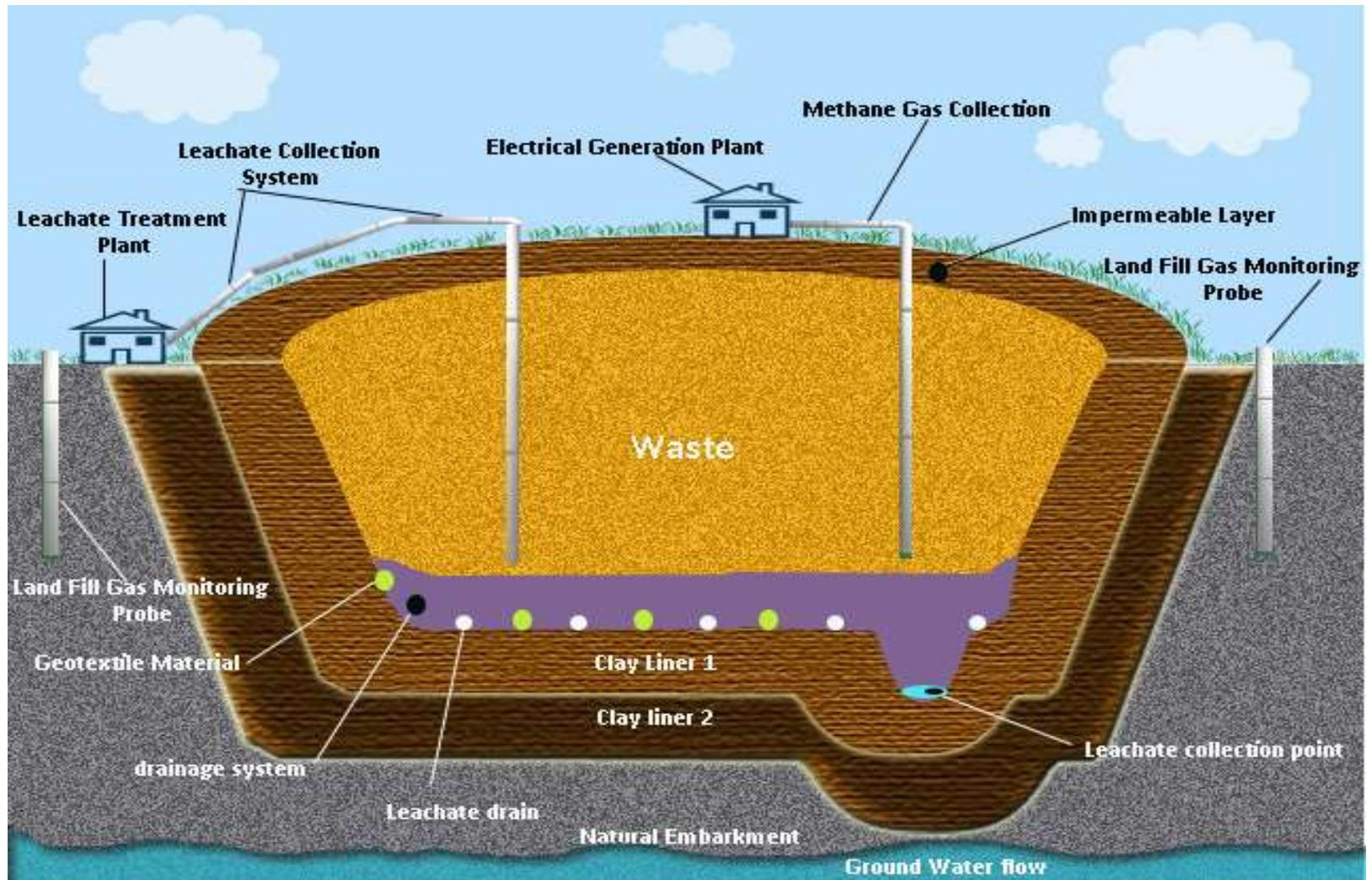
**Figure 4.23: Modern Sanitary Landfill with Two Clay Liners Proposed for High Vulnerability Area (Amadi, 2012)**
