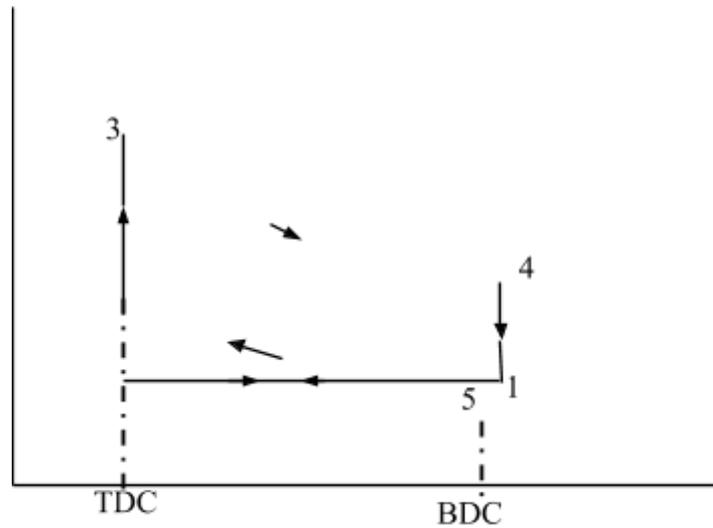
Figure 3.2: P-V diagram of six-stroke engine
