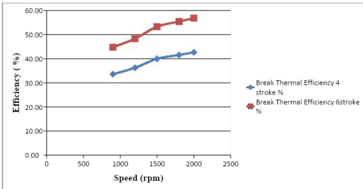
Figure 3.1: Efficiency (%) of Four-Stroke and Six-Stroke Engine
