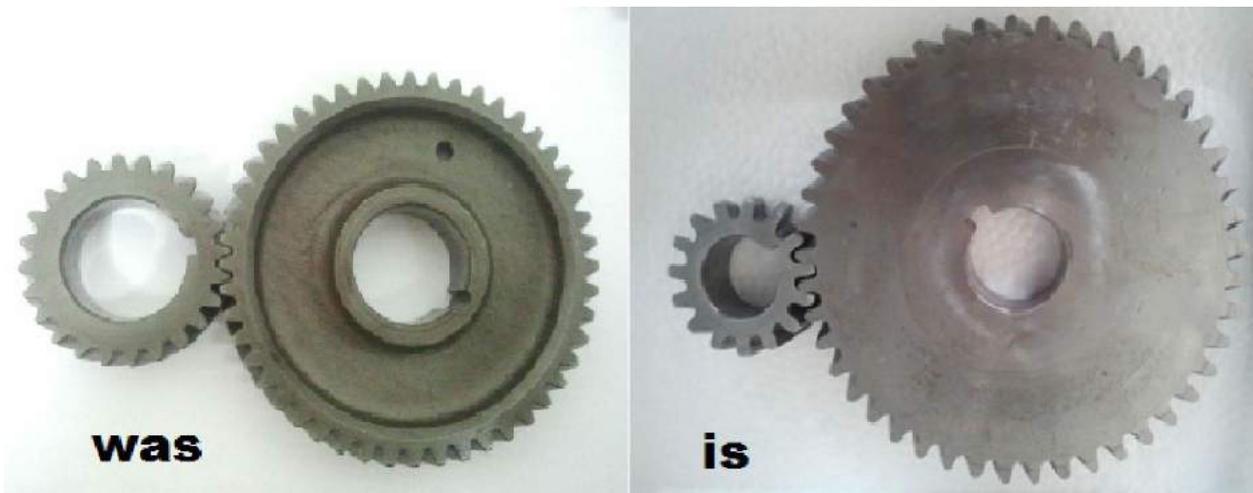
Figure 2.2: The unmodified and modified crank and cam shaft gear teeth (Shubham, 2016)
