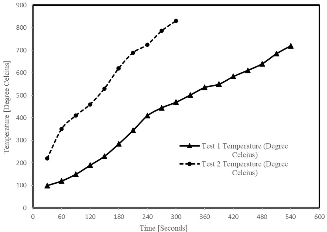
**Figure 2: Temperature-Time graph of induction furnace test**
