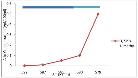
Figure 5: Effect of increase in acidic concentration using 3, 7-bis(dimethylamino) phenothiazine-5-ium chloride as modifier
