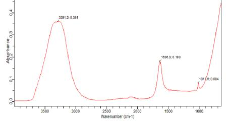
Figure 8: Infra- Red chart of dye Modified with2-(N, N-dimethyl)-4-aminophenyl as a modifier
