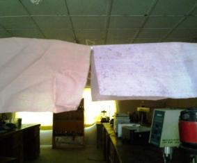
Figure 12: Effect of concentration on fixed-dye "with" a mordant and "without" a mordant at 100°C
