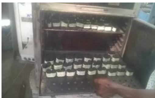
Figure 1: Composites being Oven Dried
