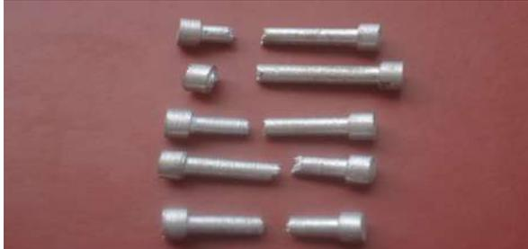
Plate I: Aluminium Cast Samples after Tensile Tests
