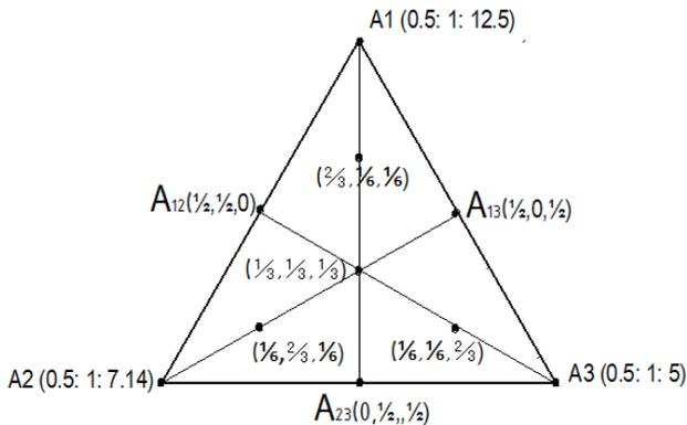
Figure 2 An augmented [3,2] Simplex lattice points for the pure, binary, control and center points
