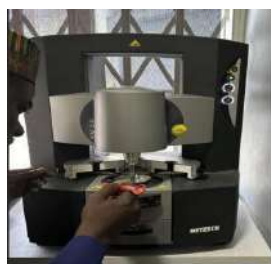
Figure 4. Loading Specimen onto the DSR machine
