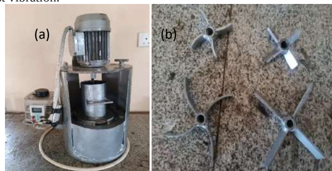
Figure 3: (a) fabricated mixer (b) fabricated impellers
