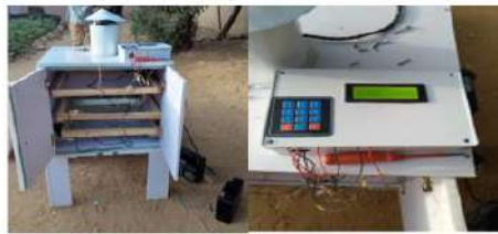
Figure 9: Designed Solar-based Dryer (Prototype)
