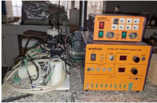
Plate 1: Armfield heat transfer service unit
