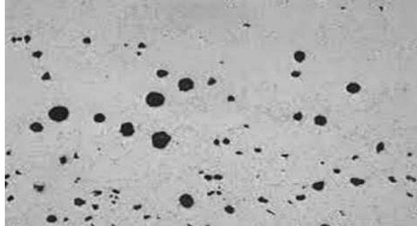
Plate 4: Porosity during deposition. (source: [1])
