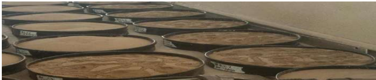
Plate II: Samples prepared for the determination of density and sediment flux.
