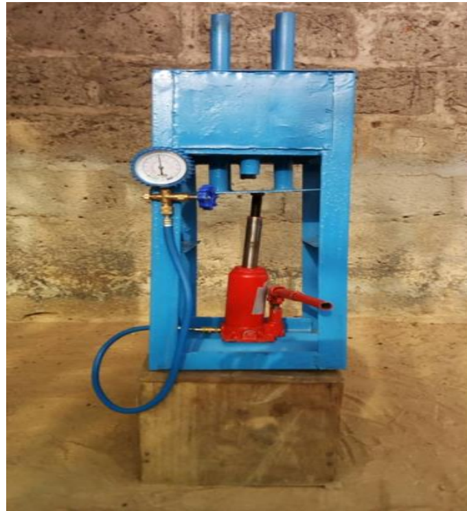
Figure 2: The fabricated briquetting machine
