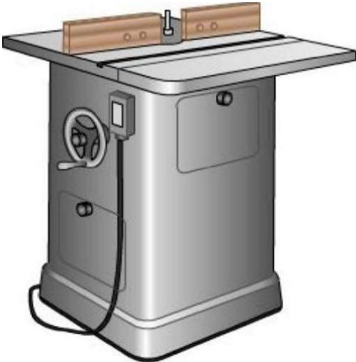
Figure 63: Light-duty shaper with adjustable fence
