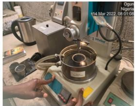
Plate VII: Penetration test in process
