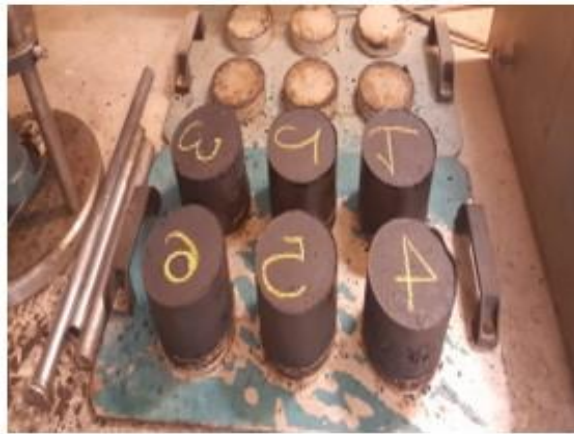
Plate V: Marshall cakes before loading on the machine
