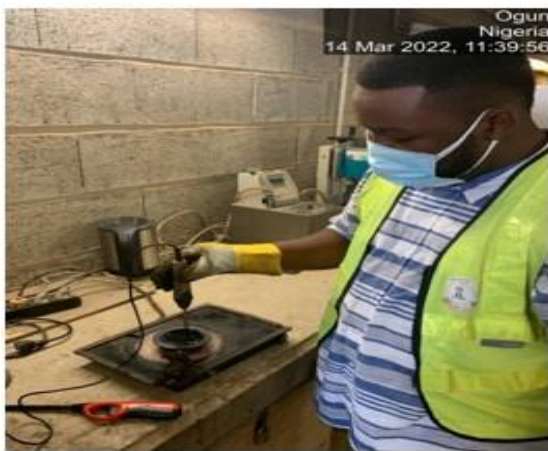
Plate VI Flash point test in process
