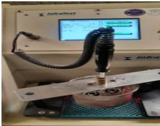
Plate IV: Softening point test in process machine
