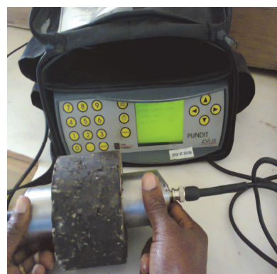
Figure 2: Rheological Test of Asphalt in progress using PUNDIT Apparatus
