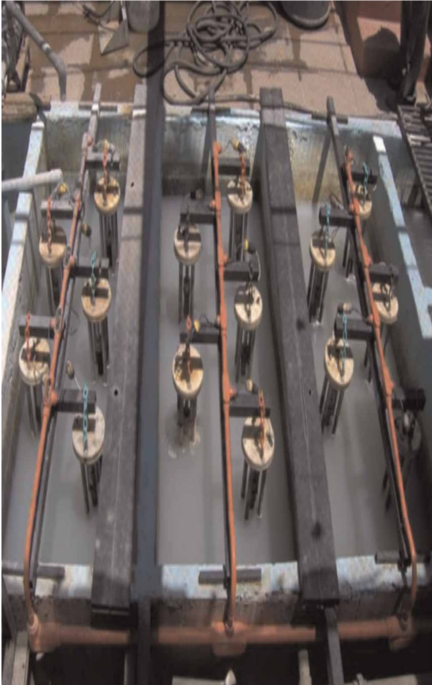
Figure 17. Picture of electroflocculation technology (copyright of Reingeniería en Saneamiento ltd).
