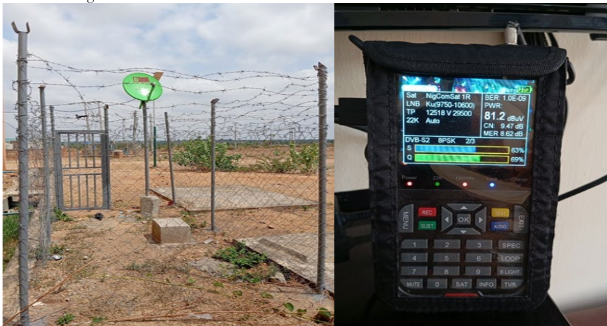
Figure 1: (a) The weather station and outdoor dish (b) The indoor digital satellite meter receiver at Federal University of Technology, Minna
