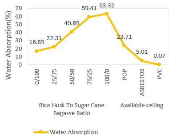
Figure 2: Water absorption test result from the composite and available ceiling
