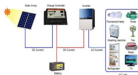
Figure 2. Diagram of a solar panel of a smart building
