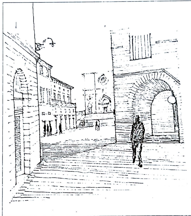
Figure 2: using different types of line to achieve 3 dimensional effects on 2 dimensional planes, Adopted from Ching (1943) pg. 115
