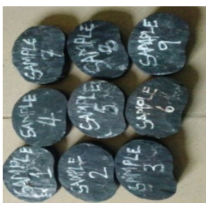
Figure 1. Produced brake pad samples.
