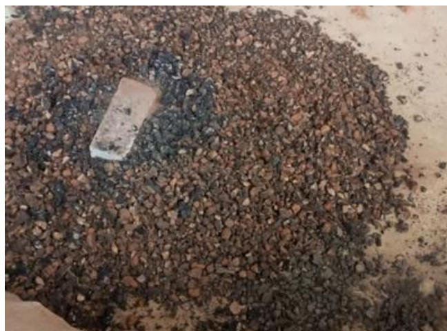
Fig. 1. Pulverized surface dressed pavement material
