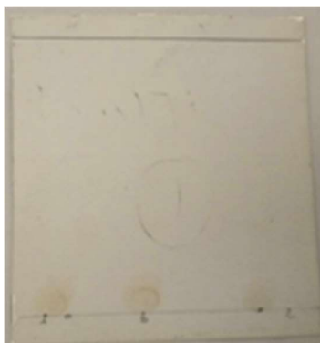
PLATE 1A: Image of the TLC chromatograph of aflatoxin produced by aflatoxigenic strain of Aspergillus flavus outside the UV hood.
