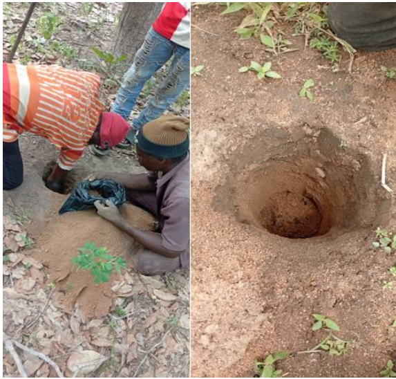
Figure 10: Residual Soil Sampling at Shallow depth of 20-50cm, dependent on soil profile
