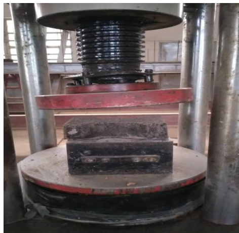
Fig. 4 Compressive strength test set up before loading starts
